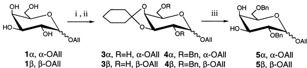
Scheme 1. (i) 1,1-Dimethylcyclohexane, H<sub>2</sub>SO<sub>4</sub>, DMF,  $\alpha$  53%,  $\beta$  71%; (ii) BnBr, KOH, Oct<sub>4</sub>NBr, CH<sub>2</sub>Cl<sub>2</sub>, 94%; (iii) HCl aq, MeOH, quant.
