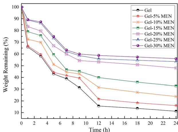
Fig. 4 Effect of macromolecule crosslinker on *in vitro* degradation of the Gel-MEN composite films.
