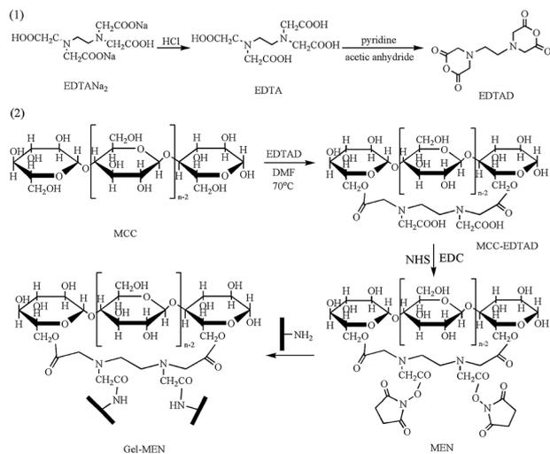
Scheme 1 The formation process of crosslinked gelatin with MEN. (1) The synthetic route of EDTA anhydride (EDTAD); (2) the preparation path of gelatin modified with MEN.
