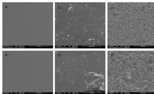
Fig. 5 Film surface morphology of Gel ( $a_1$ ,  $a_2$ ), Gel-25%MEN ( $b_1$ ,  $b_2$ ) and Gel-25%MEN after 1 h degradation ( $c_1$ ,  $c_2$ ).
