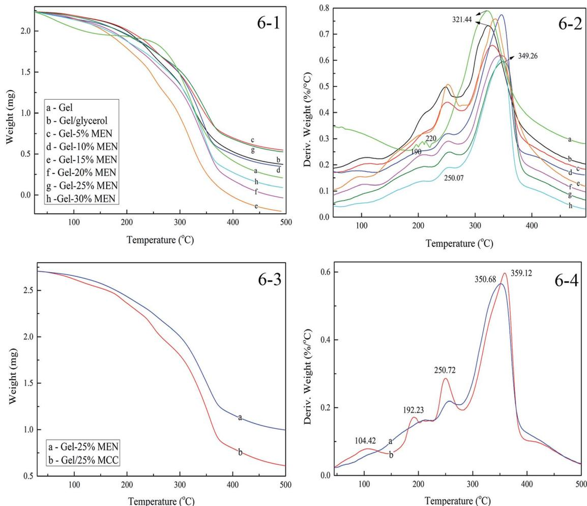
Fig. 6 TGA and DTG curves of modified gelatin films with different dosages of crosslinker (6-1 and 6-2) and comparison curves between Gel-25%MEN and Gel/25%MCC blend films (6-3 and 6-4).
