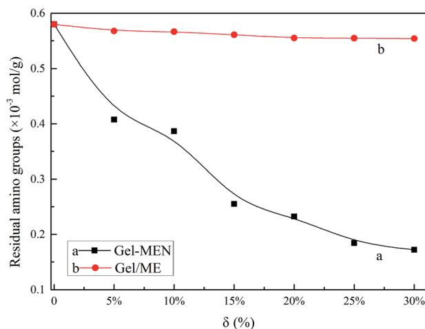
Fig. 3 Residual amino group content of gelatin solution modified with MEN (a) and ME (b) at different dosages.
