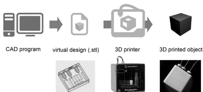
Figure 1. Fabrication of 3D-printed reactors.
