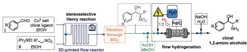
**Homemade reactors:** Stereoselective catalytic reactions were conducted in tunable homemade 3D-printed mesoreactors. This method was applied to the
