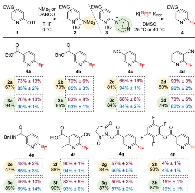
**Scheme 1.** Synthesis of precursors **2** and **3** and their radiofluorination at low temperatures. Conversions after 15 minutes at 25 or 40 °C (n = 3)
