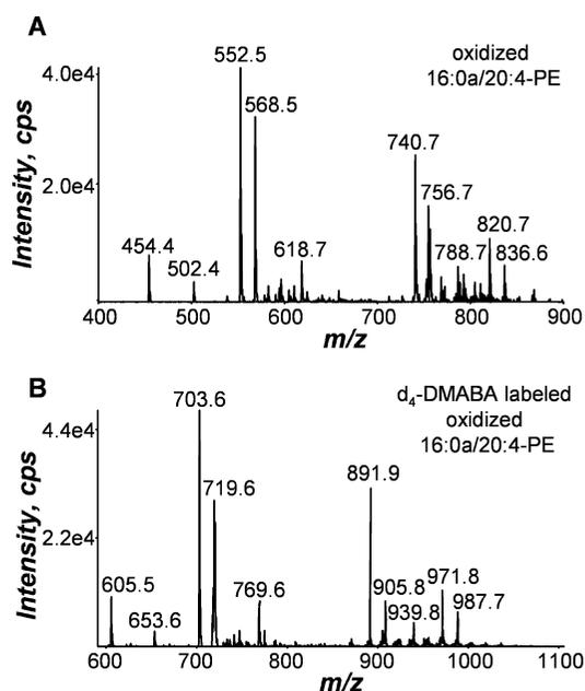
**Figure 6.** Positive ion mass spectrum of (a) oxidized 16:0a/20:4-PE and (b)  $D_4$ -DMABA labeled oxidized 16:0a/20:4-PE. Note the shift in the  $[M + H]^+$  in the  $D_4$ -DMABA labeled oxidized PE lipids by 151 amu.
