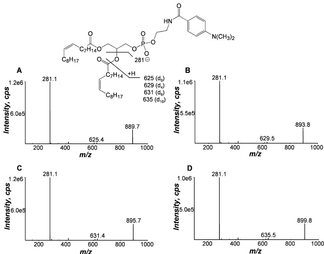
**Figure 2.** Negative ion CID spectra of the  $[M - H]^-$  of 1,2-dioleoyl-*sn*-glycero-3-phosphoethanolamine labeled with (a)  $D_0$ -DMABA NHS ester reagent, (b)  $D_4$ -DMABA NHS ester reagent, (c)  $D_6$ -DMABA NHS ester reagent, and (d)  $D_{10}$ -DMABA NHS ester reagent at a collision energy of  $-50$  V. The origins of the ions that resulted from collisional activation are indicated in the inset structure.
