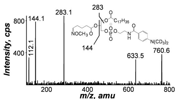
**Figure 5.** Negative ion CID of the  $[M - H]^-$  at  $m/z$  760.6 using a triple quadrupole mass spectrometer at a collision energy of  $-50$  V with a retention time of 15.41 min. The origins of the ions that resulted from collisional activation are indicated in the structures of these molecules. This data indicates that the  $[M + H]^+$  that eluted from the column at 15.41 min is MOX derivatized  $D_6$ -DMABA labeled 18:0a/5a-PE.
