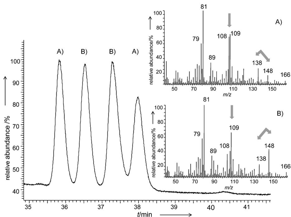
**Figure 3.** GC separation of *rac*-chrysolimidial (**1**) on a chiral Hydrodex- $\beta$ -6TBDM column along with the mass spectra of the two diastereomeric pairs (*5R,8S*),(*5S,8R*) and (*5R,8R*),(*5S,8S*). The two diastereomeric pairs display different, but significant relative intensities of the ions at  $m/z$  108 and 109, or at  $m/z$  148 and 138. Elution order: A) (*5R,8S*), 35.8 min, (*5S,8R*) 38.0 min. B) (*5R,8R*) 36.5 min, (*5S,8S*) 37.3 min.
