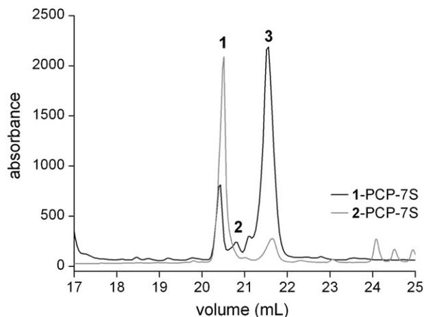
**Figure 5.** HPLC chromatograms showing peptide hydrazide products of OxyB reaction following hydrazine cleavage using 1-PCP-7S (black) and 2-PCP-7S (gray) as substrates. Peak 1, monocyclic product (**4**); peak 2, unreacted linear peptide; peak 3, monocyclic product (**3**) (see Fig. 3).
