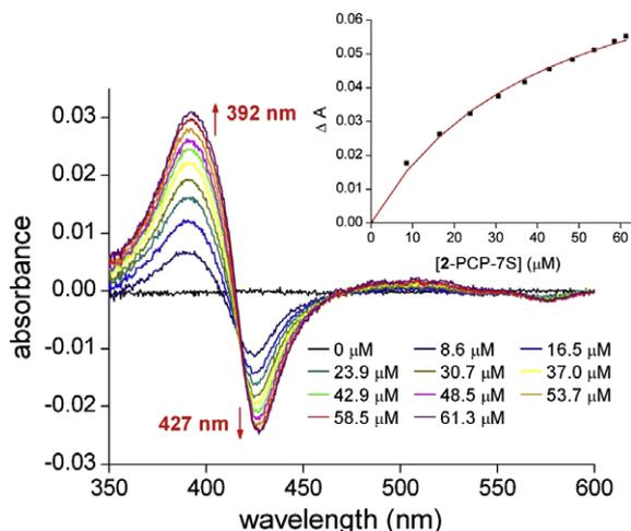
**Figure 6.** Difference UV-vis spectra of hexapeptide **2-PCP-7S** binding to OxyB. The concentration dependence of the spectral changes and the wavelengths of the minima and maxima are shown.
