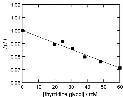
**Figure 3.** Relative intensity of fluorescence of FMN (0.1 mM) at 520 nm upon excitation at 370 nm in the presence of adenosine (15 mM) and various concentrations of thymidine glycol (0–60 mM) in deoxygenated phosphate buffer (pH 7.0).
