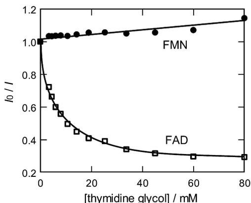
**Figure 1.** Stern–Volmer plots for fluorescence quenching of (●) FMN and (□) FAD by thymidine glycol. Relative intensity ( $I_0/I$ ) of the emission at 520 nm was measured in the presence of 0.1 mM flavin in deoxygenated phosphate buffer solution (pH 7.0).
