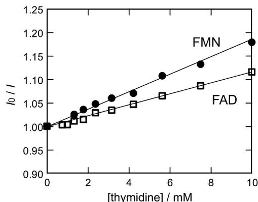
**Figure 2.** Stern–Volmer plots for fluorescence quenching of (●) FMN and (□) FAD by thymidine. Upon excitation at 370 nm, relative intensity ( $I_0/I$ ) of the emission at 520 nm was measured in the presence of 0.1 mM flavin in deoxygenated phosphate buffer solution (pH 7.0).
