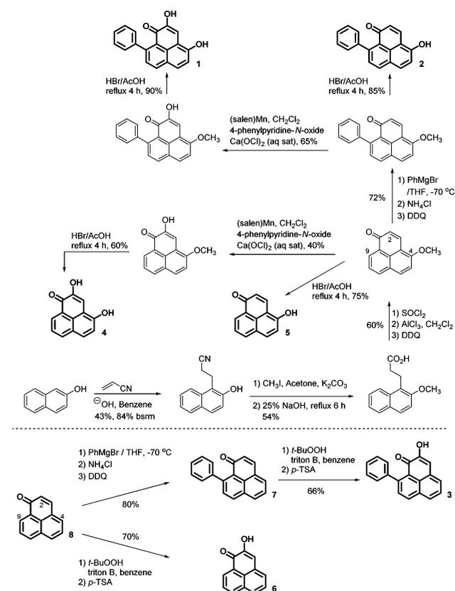
Scheme 1 illustrates the synthetic sequence for the preparation of the required compounds. This scheme shows previously reported procedures which produced already characterized products (except compounds **2** and **4**, see Supporting Information).<sup>9,11</sup> In brief, refluxing acrylonitrile with a basic solution of 2-naphthol afforded the corresponding propanenitrile. This compound was subjected
