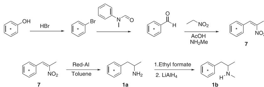
**Scheme 1.** Synthesis of  $[^{13}\text{C}_6]$ -amphetamine (**1a**) and  $[^{13}\text{C}_6]$ -methamphetamine (**1b**). \*All aromatic carbons as  $^{13}\text{C}$ .
