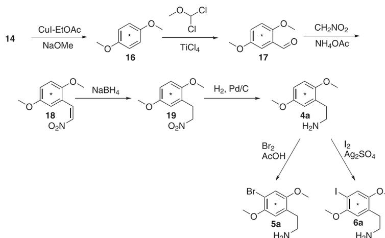
**Scheme 4.** Synthetic route to the [ $^{13}\text{C}_6$ ]-labelled derivatives **4a**, **5a** and **6a**. \*All aromatic carbons as  $^{13}\text{C}$ .
