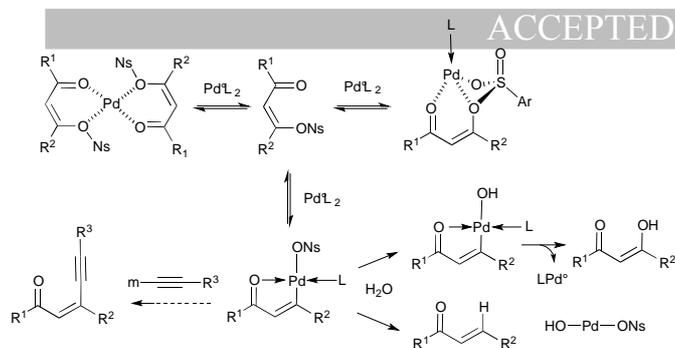
**Scheme 3.** Possible explanations for the lack or poor reactivity of *Z*- $\beta$ -keto nosylates.
