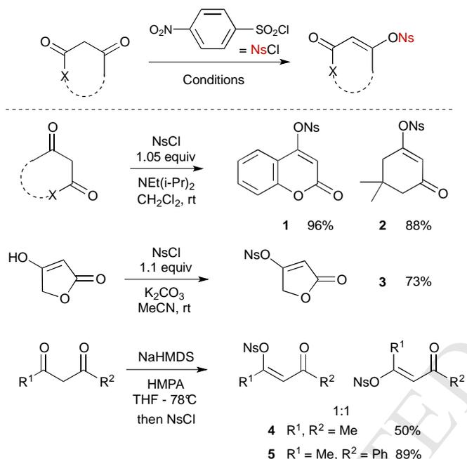
**Scheme 2.** Standard procedures for the preparation of vinyl nosylate derivatives **1-5** using NsCl.
