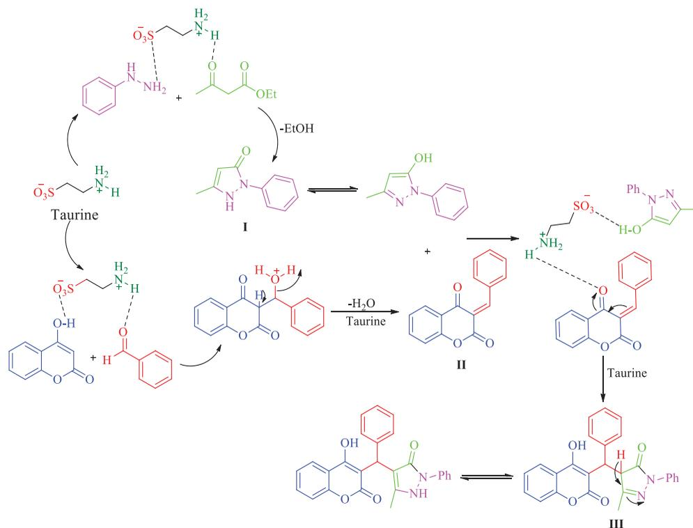
**Scheme 4.** A possible mechanism for the formation of benzylpyrazolyl coumarin.
