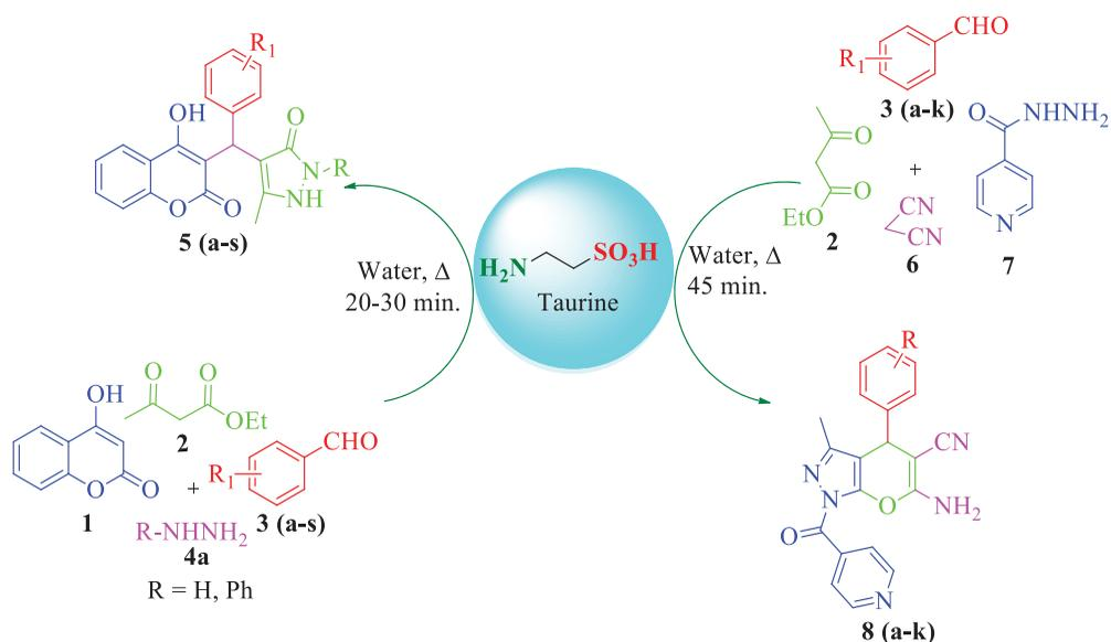
**Scheme 1.** General scheme for the synthesis of benzylpyrazolyl coumarin **5 (a-s)** and novel 6-amino-1-isonicotinoyl-3-methyl-4-phenyl-1,4-dihydroprano[2,3-c]pyrazole-5-carbonitrile derivatives **8 (a-k)**.
