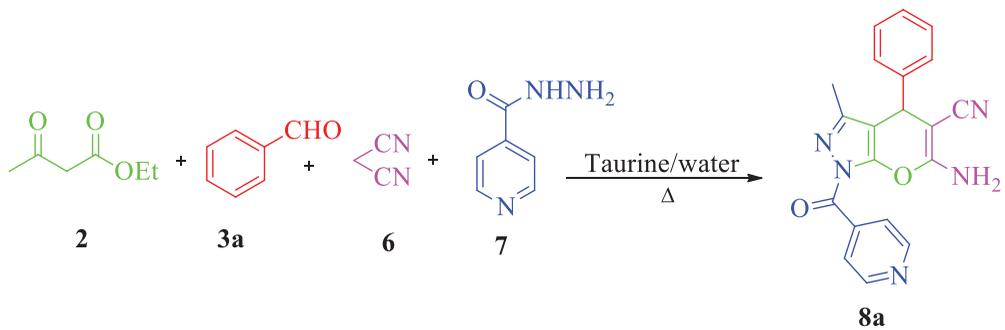
**Scheme 3.** Synthesis of pyrano[2,3-c]pyrazole-5-carbonitrile.
