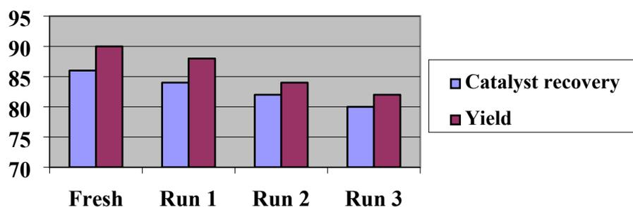
**Figure 2.** Reuse and recovery of  $\beta$ -CD and its effect on yield
