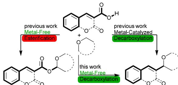
**Scheme 3.** Decarboxylation versus Esterification in the presence and absence of metals.
