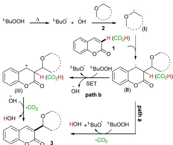
**Scheme 4.** Proposed mechanism of TM-free alkylation of coumarins/coumarin carboxylic acids.
