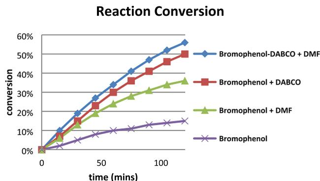
**Figure 2.** Impact of DABCO on reaction conversion.
