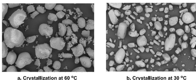
**Figure 1.** Controlling bromophenol-DABCO crystal particle size through temperature.
