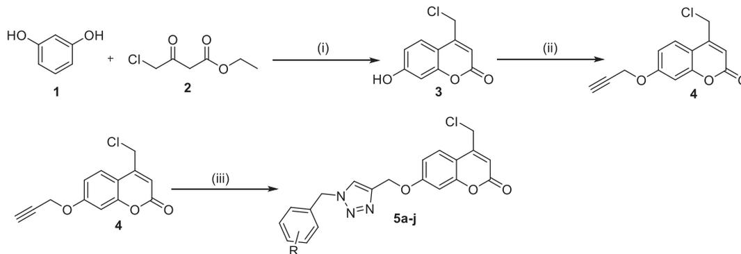
**Scheme 2.** Synthesis of coumarin-linked triazoles (**5a-j**)-Reagents and conditions: (i) H<sub>2</sub>SO<sub>4</sub>, ice bath, 15 min, 95% (ii) Propargyl bromide, K<sub>2</sub>CO<sub>3</sub>, acetone, rt, 3–4 h 90% (iii) Substituted benzyl azides, CuSO<sub>4</sub>·5H<sub>2</sub>O, sodium ascorbate, EtOH:H<sub>2</sub>O::1:1, rt, overnight, 72–90%.
