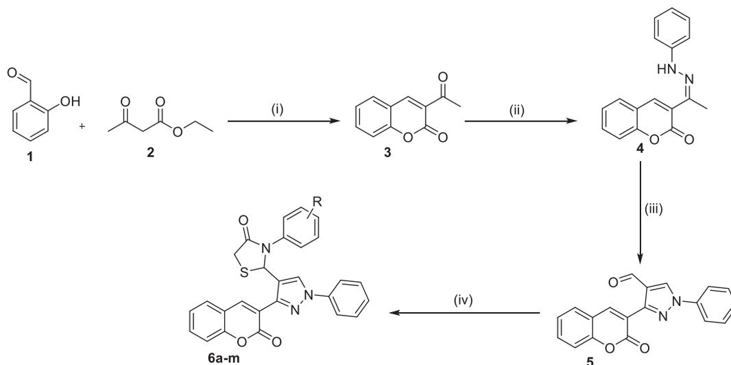
**Scheme 1.** Synthesis of coumarin linked 4-thiazolidinones via pyrazole linker (**6a-m**)-Reagents and conditions: (i) Catalytic piperidine, neat, 90% (ii) Phenylhydrazine, Glacial acetic acid, rt, 30 min, 95% (iii) DMF/POCl<sub>3</sub>, 0 °C-rt, 24 h, 73% (iv) Substituted anilines, thioglycolic acid, silica gel (100–200 mesh), DCM, rt, 3–12 h, 42–64%.
