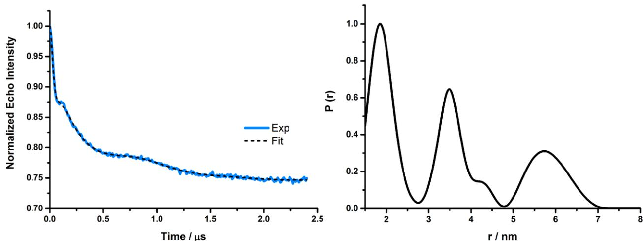
Figure 2. PELDOR measurement of 12mer-duplex-RNA **17** at Q-band frequency. (a) Background-corrected PELDOR trace (in blue) and Tikhonov regularization (in black) by using DEER analysis.<sup>[15]</sup> (b) Calculated distance distribution with an overall maximum at 1.85 nm. Peaks at around 3.5 and 5.7 nm correspond to intermolecular distances due to stacking of RNA molecules. Data was normalized and a regularization parameter  $\alpha$  of 10 was used.
