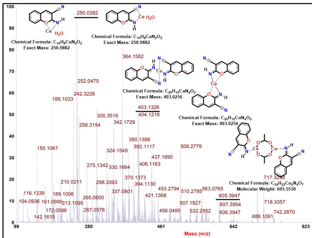
**Figure 4.** MALDI-ESI mass spectra (2, 4-Dihydroxybenzoic acid as the matrix) of  $\text{Cu}(\text{OAc})_2 \cdot \text{H}_2\text{O}$  and 2-imino-2H-chromene-3-carbonitrile stirred at room temperature in 2-MeTHF solvent for 24 h.
