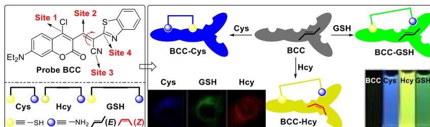
A multi-signal fluorescent probe was exploited for simultaneously distinguishing and sensing of cysteine, homocysteine and glutathione in living cells.
