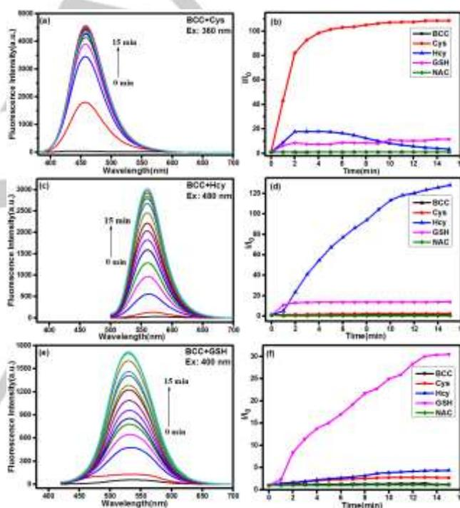
**Figure 2.** Time-dependent fluorescence spectra of **BCC** (10  $\mu$ M) in the presence of (a) 10 equiv. of Cys excited at 360 nm, (c) 10 equiv. of Hcy excited at 480 nm, (e) 10 equiv. of GSH excited at 400 nm, respectively. Time-dependent fluorescence intensity changes toward 10 eq. of biothiols excited at (b) 360 nm, (d) 480 nm and (f) 400 nm respectively. Condition: DMSO-PBS (pH 7.4, 10 mM, v/v, 6/4) at room temperature. Slit (nm): 2.5/2.5.
