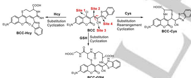
**Scheme 2.** Proposed mechanisms of probe **BCC** with Cys, Hcy and GSH.
