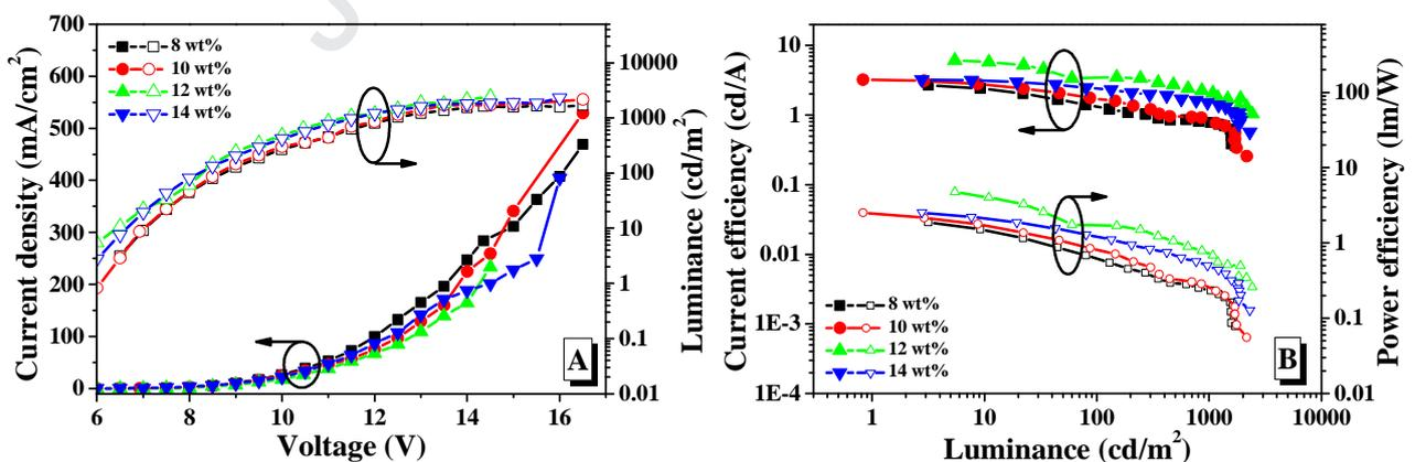
Fig. 8. (A) Luminance-voltage-current density ( $L-V-J$ ) characteristics and (B) current/power efficiency versus luminance curves of the devices based on **PI-C** with different dopant concentrations.
