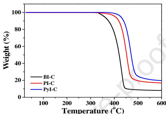
Fig. 1. Thermogravimetric analyses (TGA) of **BI-C**, **PI-C** and **PyI-C** in nitrogen atmosphere (heating rate: 10 °C/min).
