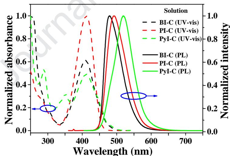
Fig. 2. UV-vis absorption and photoluminescence spectra of the compounds **BI-C**, **PI-C** and **PyI-C** in dichloromethane solutions ( $C = 1.0 \times 10^{-5}$  mol/L).
