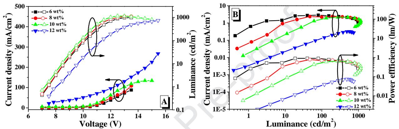
Fig. 7. (A) Luminance-voltage-current density ( $L-V-J$ ) characteristics and (B) current/power efficiency versus luminance curves of the devices based on **BI-C** with different dopant concentrations.
