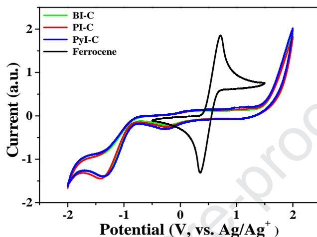
Fig. 4. Cyclic voltammograms of ferrocene and the compounds **BI-C**, **PI-C** and **PyI-C** (scan rate: 10 mV/s; solvent: dichloromethane).
