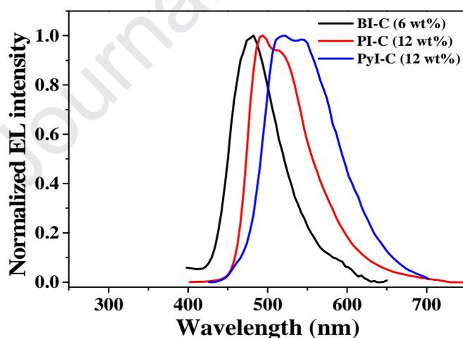
Fig. 10. EL spectra of the devices based on the compounds with maximum luminous efficiencies.
