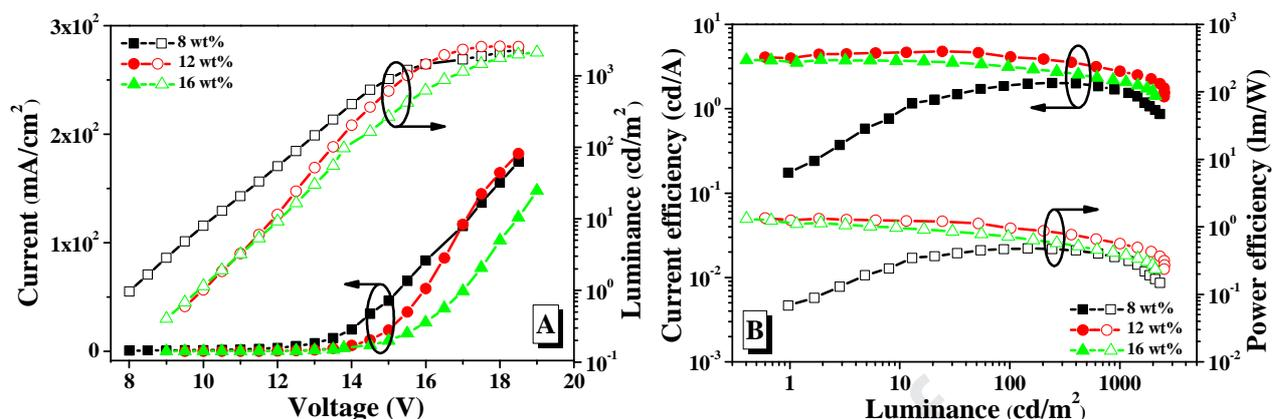
Fig. 9. (A) Luminance-voltage-current density ( $L-V-J$ ) characteristics and (B) current/power efficiency versus luminance curves of the devices based on **PyI-C** with different dopant concentrations.
