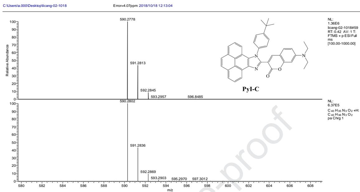
Fig. S9. Mass spectrum of PyI-C
