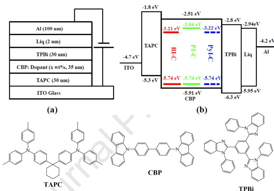
Fig. 6. Schematic diagram of the OLED device configuration (a), the relative HOMO/LUMO energy levels of the materials investigated in this work (b) and structures of TAPC, CBP and TPBi (bottom).
