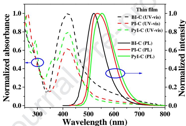
Fig. 3. UV-vis absorption and photoluminescence spectra of the compounds **BI-C**, **PI-C** and **PyI-C** in the solid films.
