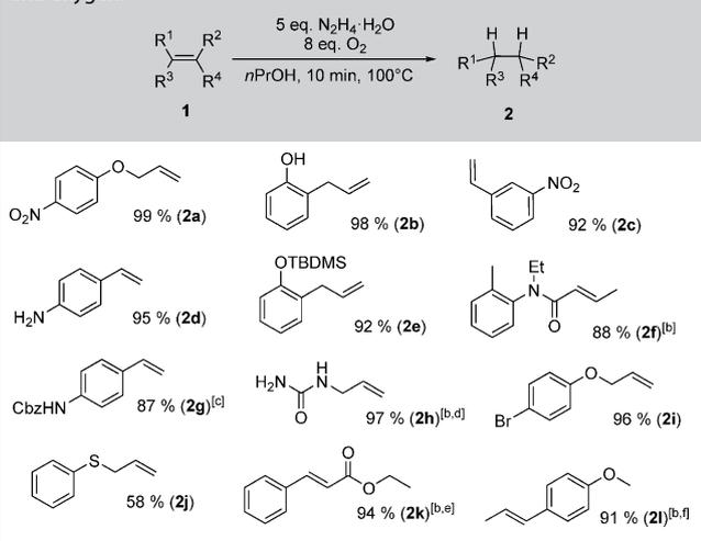
[a] Conditions: Olefin (0.5 M) and hydrazine hydrate (4 equiv) in *n*PrOH, 0.4 mL min<sup>-1</sup> liquid flow rate, 40 mL min<sup>-1</sup> O<sub>2</sub> flow rate, 20 bar back pressure, 10 mL PFA coil. [b] 5 equivalents of hydrazine hydrate were used. [c] conc. = 0.33 M. [d] *n*PrOH/H<sub>2</sub>O (1:1 v/v) as solvent. [e] Reaction was carried out at 120 °C in a 16 mL coil. [f] Reaction was carried out at 120 °C in a 26 mL coil.
