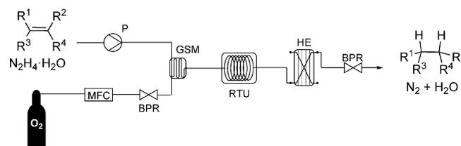
Figure 1. Two-feed continuous-flow setup for the reduction of olefins with diimide.
