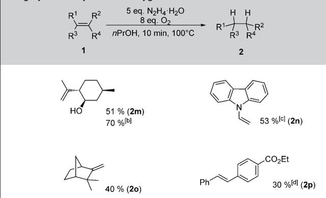
[a] Conditions: Olefin (0.5 M) and hydrazine hydrate (4 equiv) in *n*PrOH, 0.4 mL min<sup>-1</sup> liquid flow rate, 40 mL min<sup>-1</sup> O<sub>2</sub> flow rate, 20 bar back pressure, 10 mL PFA coil. Conversions determined as GC-FID peak area percent. [b] Reaction was carried out at 120 °C in a 26 mL coil. [c] Toluene/*n*PrOH (3:7 v/v) was used as solvent. [d] 0.1 M in toluene/*n*PrOH (3:2 v/v).
