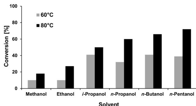
**Figure 2.** Solvent screening for the continuous reduction of allylbenzene using 5 equivalents of hydrazine hydrate in presence of oxygen.
