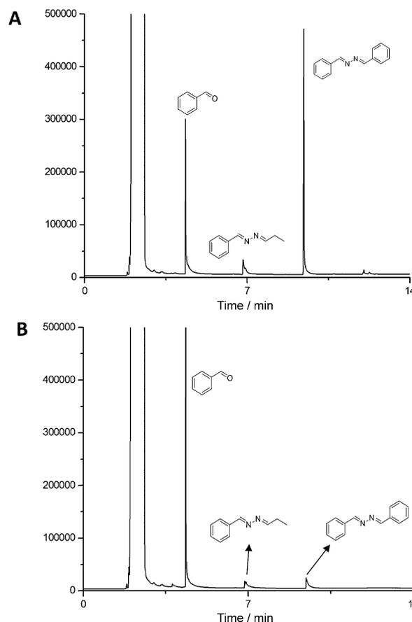
**Figure 4.** GC-MS chromatograms from the benzaldehyde trapping experiments using a 2.5 (A) or a 5.5 mL coil (B) for the oxidation of hydrazine and diimide oxidation/disproportionation.
