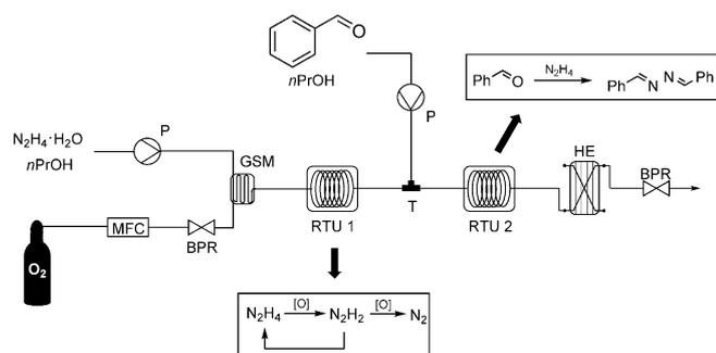
**Figure 3.** Continuous-flow setup for the hydrazine trapping experiments using benzaldehyde.
