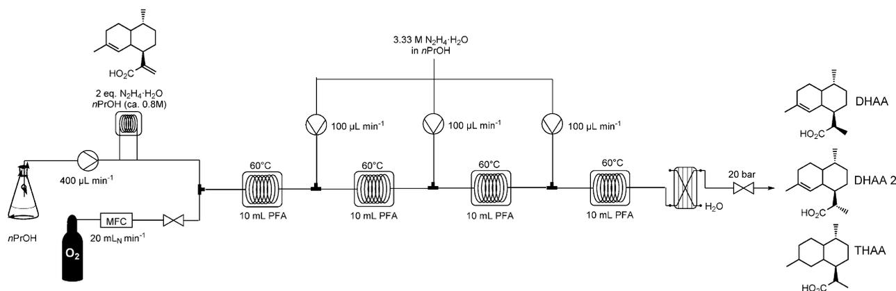
**Figure 5.** Optimized multi-injection setup for the reduction of artemisinic acid towards in situ generation of diimide from hydrazine hydrate and oxygen.
