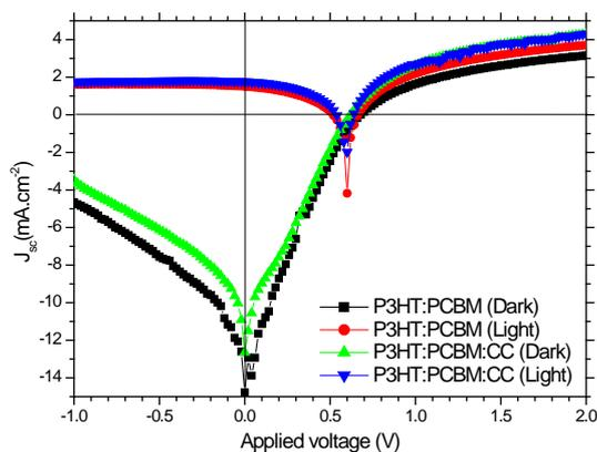
Figure 10. The  $J(V)$  characteristics of the pristine P3HT:PCBM and P3HT:PCBM:CC-based OSCs.
