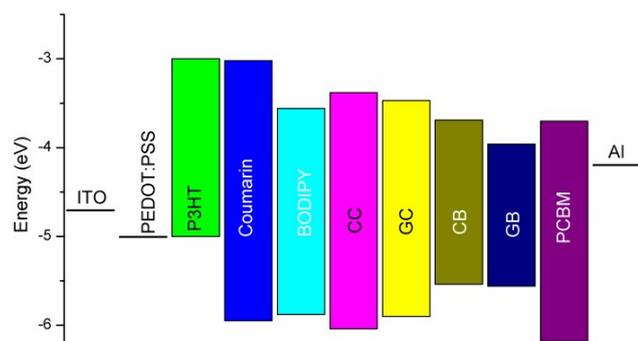
Figure 5. Determined energy diagram with HOMO/LUMO levels of coumarin, BODIPY, CC, GC, CB and GB in a BHJ OSC device
