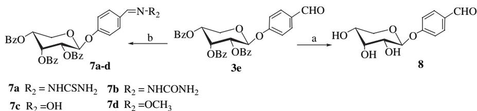
Scheme 4. Preparation of **7a–d** and **8**. Reagents and conditions: (a) NaOMe, MeOH, rt, 12 h; (b) amine, EtOH, reflux or 45 °C, 2–6 h.
