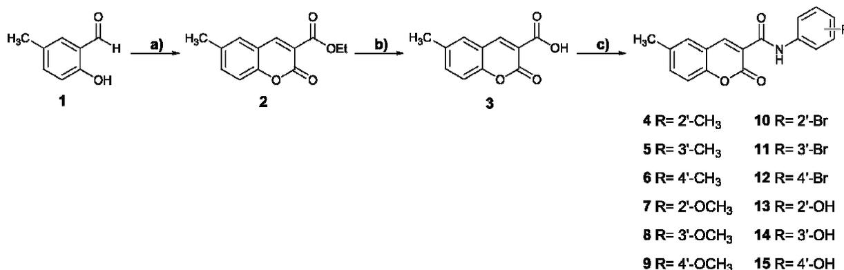
Scheme 1 - Synthesis of coumarins **4-15**. Reagents and conditions: a) diethyl malonate, EtOH, piperidine, reflux, overnight. b) NaOH (0.5% aq./EtOH), reflux, 4h. c) EDC, DMAP, DCM, corresponding amine, 0  $^{\circ}$ C to r.t., 4h.
