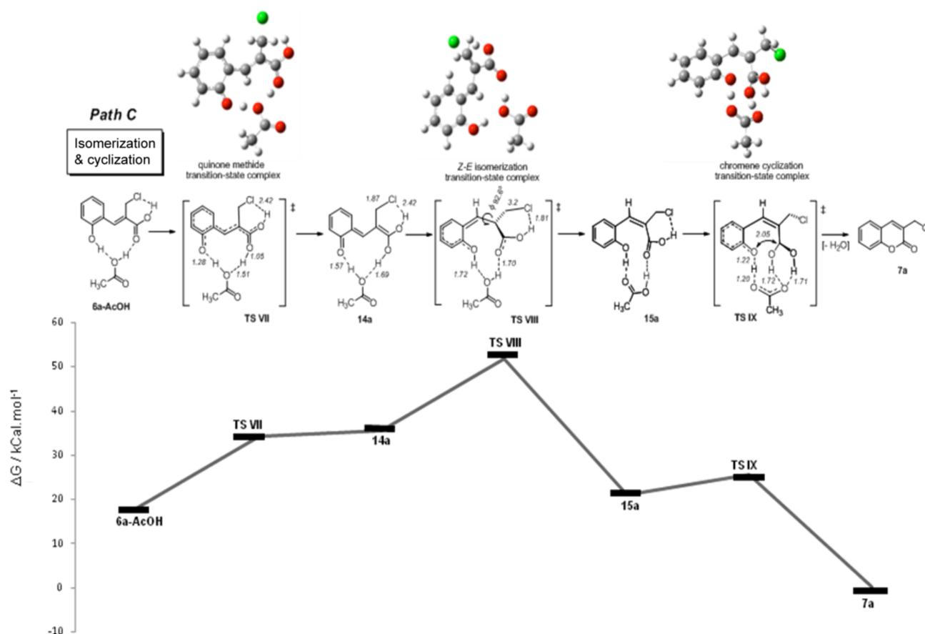
**Figure 11.** Mass-balanced free energy profile for the *Z*–*E* isomerization of 2-(chloromethyl)cinnamic acid derivative **6a** and subsequent cyclization to give 3-(chloromethyl)coumarin **7a** (path C), showing ball-and-stick structures for the transition states TS IV–TS VI, colored according to atom type (H, white; C, gray; O, red; Cl, green).
