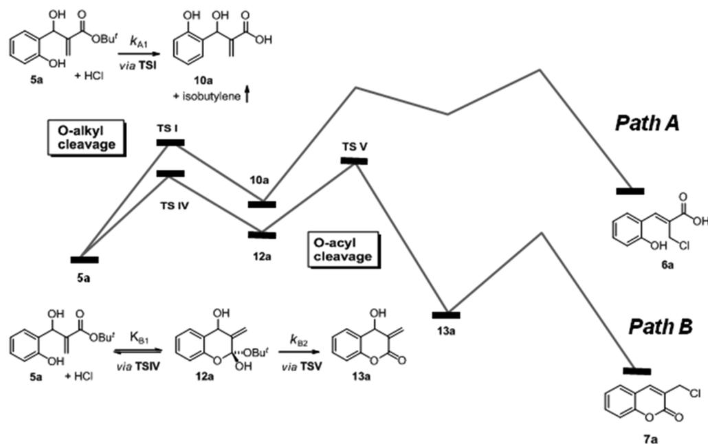
**Figure 10.** Superimposed mass-balanced free energy profiles for the formation of the major product **6a** via *O*-alkyl cleavage (path A) and the minor product **7a** via *O*-acyl cleavage (path B).
