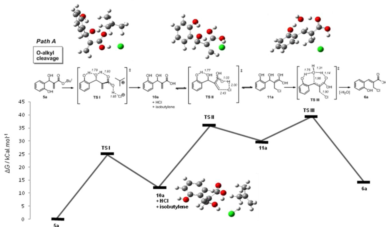
**Figure 8.** Mass-balanced free energy profile for the formation of the major product **6a** via O-alkyl cleavage (path A), showing ball-and-stick structures for the transition states TS I–TS III and the stable arrangement of the three discrete species **10a**, isobutylene, and HCl, colored according to atom type (H, white; C, gray; O, red; Cl, green).
