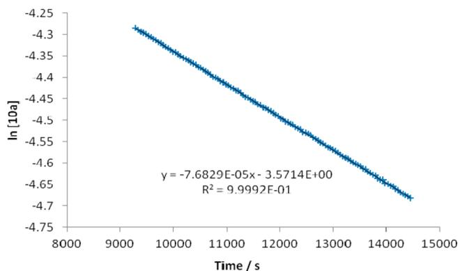
**Figure 4.** Logarithmic pseudo-first-order kinetic plot from 9000 s onward reflecting the consumption of intermediate **10a** leading to the major product **6a** at 286.45 K;  $[\text{HCl}] = 2.35 \text{ M}$ .
