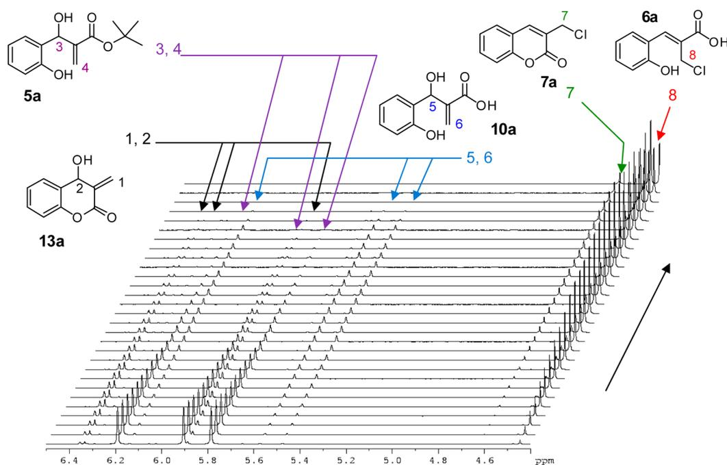
**Figure 2.** Partial time-dependent 600 MHz  $^1\text{H}$  NMR spectra selected at 300 s intervals from the commencement of the reaction of the Baylis–Hillman adduct **5a** with in situ-generated HCl in methanol- $d_4$  at 276.2 K, illustrating some of the signals assigned to structures **5a**, **6a**, **7a**, **10a**, and **13a**.
