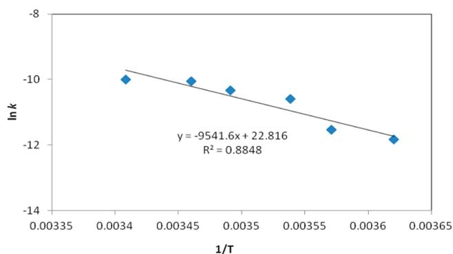
**Figure 5.** Arrhenius plot ( $\ln k$  against  $1/T$ ) for the consumption of intermediate **10a** leading to the major product **6a**.
