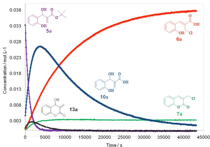
**Figure 7.** Plots of concentrations against time (from 600 MHz  $^1\text{H}$  NMR spectra in methanol- $d_4$ ) for the reaction of the Baylis–Hillman adduct **5a** with in situ-generated HCl at 276.2 K, showing the consumption of the substrate and the formation of intermediates **10a** and **13a**, the major product **6a**, and the minor product **7a**.
