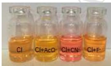
**Fig. 7.** Photographs of **CT-1** ( $c=2 \times 10^{-5}$  M in DMSO/H<sub>2</sub>O (9:1)) upon addition of 20 equiv of F<sup>-</sup>, AcO<sup>-</sup> and CN<sup>-</sup> ( $c=1 \times 10^{-5}$  M in DMSO) under ambient light.
