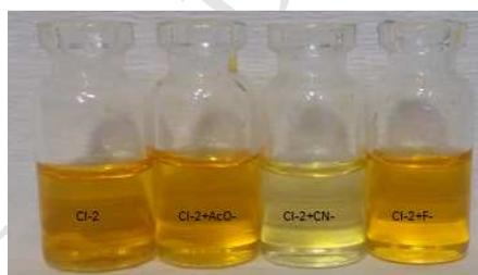
**Fig. 9.** Photographs of **CI-2** ( $c=2\times 10^{-5}$  M in DMSO) upon addition of 20 equiv of  $\text{F}^-$ ,  $\text{AcO}^-$  and  $\text{CN}^-$  ( $c=1\times 10^{-5}$  M in DMSO) under ambient light.
