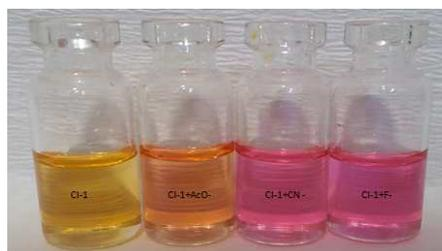
**Fig. 4.** Photographs of **CI-1** ( $c=2\times 10^{-5}$  M in DMSO) upon addition of 20 equiv studied anions ( $c=1\times 10^{-2}$  M in DMSO) under ambient light.
