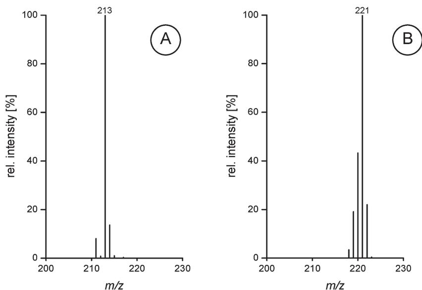
**Figure 2.** Mass spectra (MS-CI) of 12-methyltridecanal (A) and [ $^2\text{H}_8$ ]-12-methyltridecanal (B).
