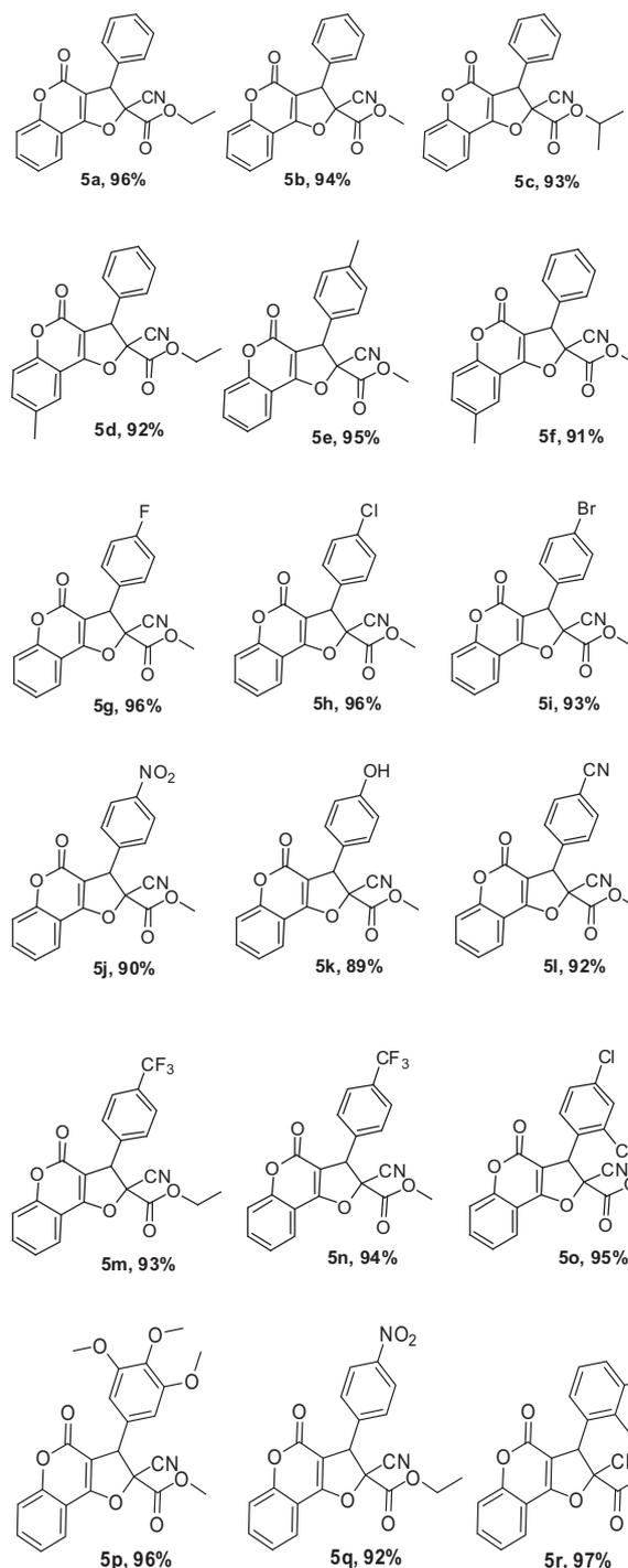
**Scheme 3.** Reaction conditions: 4-hydroxy coumarin (**1**, 2.8 mmol), benzaldehyde (**2**, 2.8 mmol) and malanonitrile (**3**, 2.8 mmol) in 5 mL ethanol at 80 °C temperature about 1 h and then added NCS (**4**, 2.8 mmol) rt 15 min. Yields refers to pure products.
