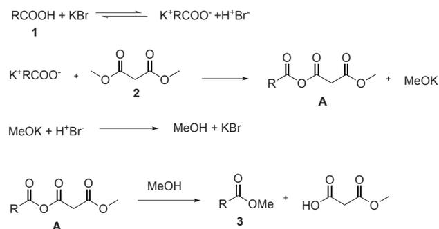
**Scheme 6.** A proposed mechanism for DMM-mediated methylation.
