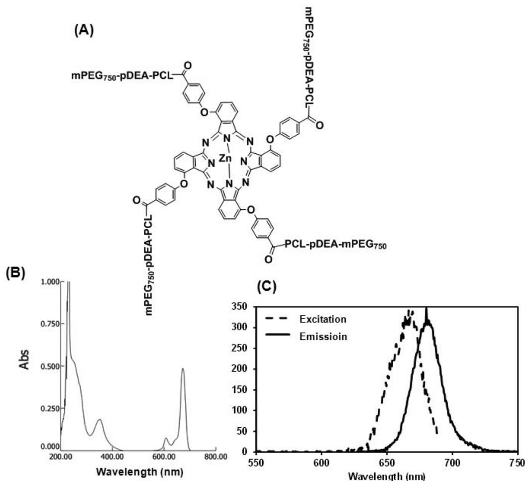
**Figure 2.** Properties of PDCZP. (A) Molecular structure of PDCZP. (B) The UV-vis absorption spectrum of PDCZP solutions in THF. (C) Fluorescent excitation and emission spectra of PDCZP solutions in DMF.
