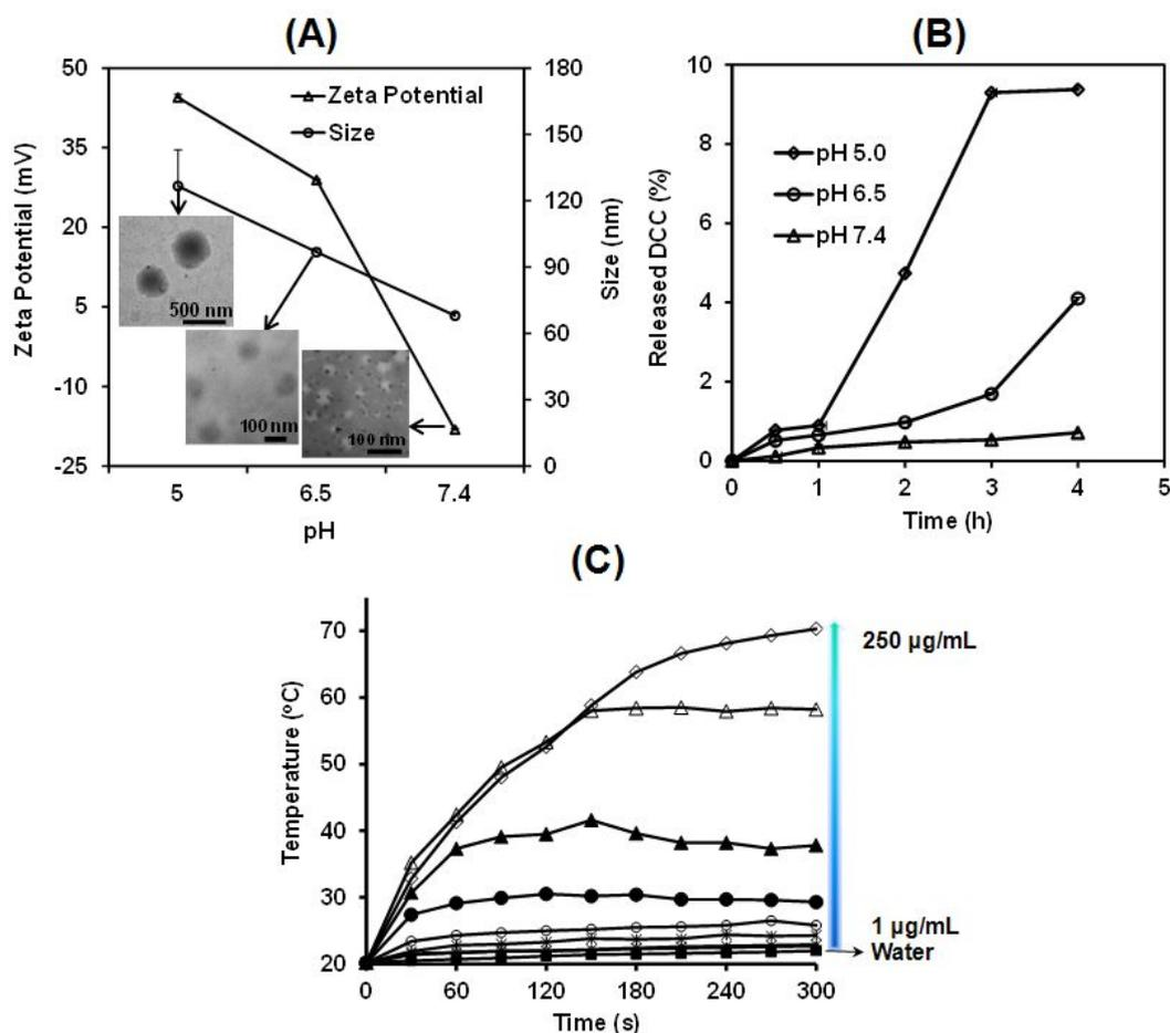
**Figure 3.** Properties of DCC@PDCZP. (A) Size and zeta potential of DCC@PDCZP and the corresponding TEM images with pH dependency ( $n = 3$ ). (B) DCC release from DCC@PDCZP with pH dependency ( $n = 3$ ). (C) Temperature profiles of
