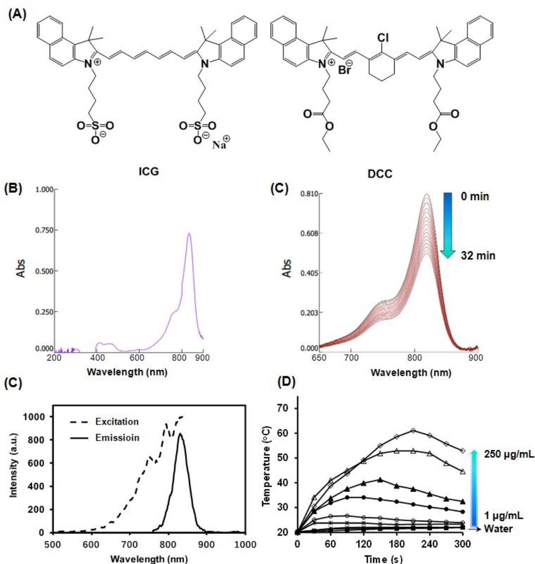
**Figure 1.** Molecular structures of ICG and DCC (A), and properties of DCC. (B) the UV-vis spectrum of DCC solutions in methanol. (C) Visible absorption spectral changes of DCC solutions in methanol with time dependency. (D) Fluorescent excitation and emission spectra of DCC solutions in DMSO. (E) Temperature profiles of DCC aqueous suspensions after 830 nm and 1.0 W/cm<sup>2</sup> light irradiation with concentration dependency.
