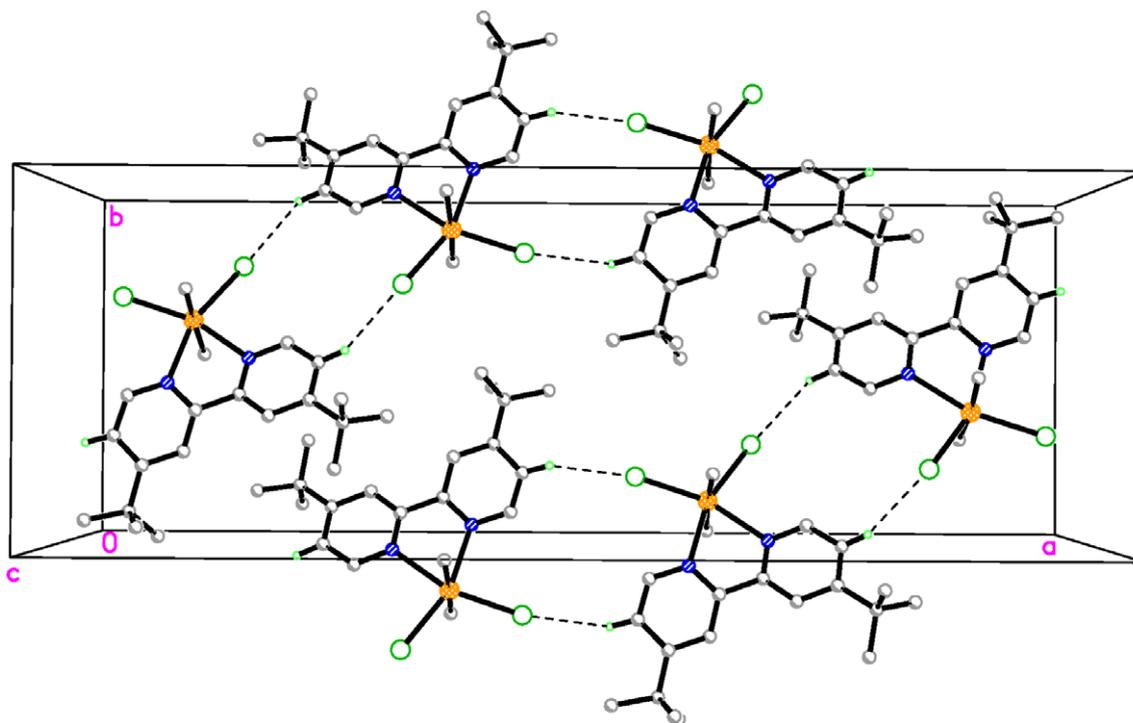
**Fig. 2.** The crystal packing of complex **1a**, viewed down the *c*-axis, showing linking of the neighboring molecules through intermolecular C–H...Cl interactions along the *a*-axis. The H-atoms except those involved in interactions are omitted for clarity. Intermolecular interactions are shown as dashed lines.
