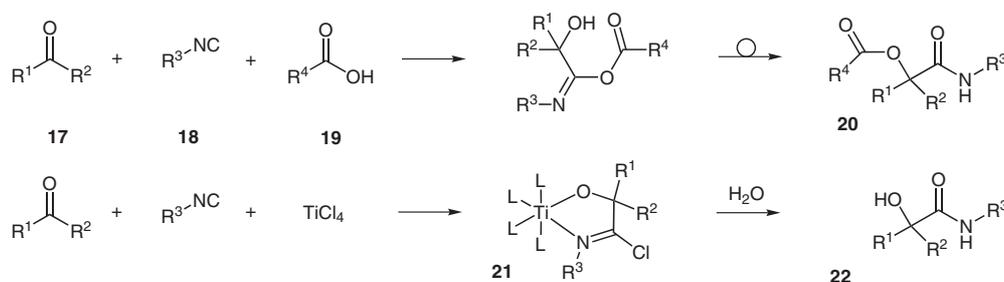
**Scheme 5** Classical Passerini reaction versus titanium tetrachloride assisted Passerini reaction (L = Cl or donor group of substrate)
