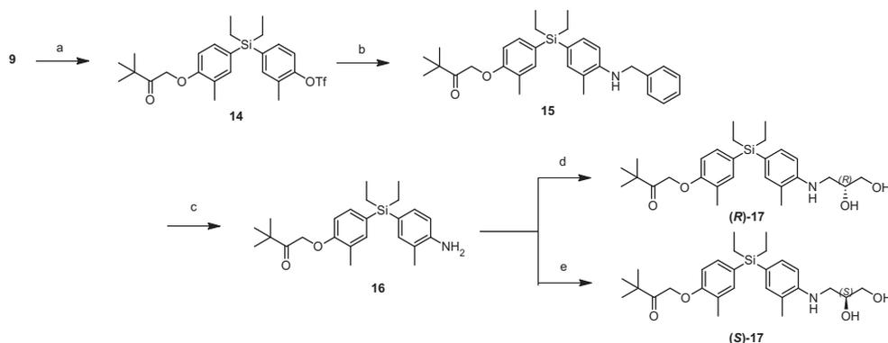
**Scheme 4.** Synthesis of the aza-analogs (*R*)-**17** and (*S*)-**17**. Reagents and conditions: (a) triflic anhydride, triethylamine, CH<sub>2</sub>Cl<sub>2</sub>, rt, 1 h, 88%; (b) palladium diacetate, BINAP, Cs<sub>2</sub>CO<sub>3</sub>, benzylamine, toluene, 100 °C, 6 h, 72%; (c) Pd/C, H<sub>2</sub>, EtOH, 61%; (d) (*S*)-glycidol, ethanol, 75 °C, 11 h, 42%; (e) (*R*)-glycidol, ethanol, 75 °C, 11 h, 47%.
