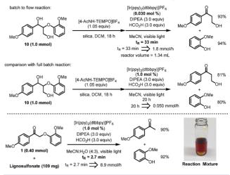
no conversion after 48 h. However, when the same reaction was carried out in flow, we observed full consumption of 1, providing a high yield of both guaiacol and 4'-methoxyacetophenone, despite reduced light transmittance (Scheme 2). This clearly demonstrates the ability of our reaction to operate in the presence of sulfonate groups, solvent quantities of water, and dark colored impurities found in lignosulfonate.
