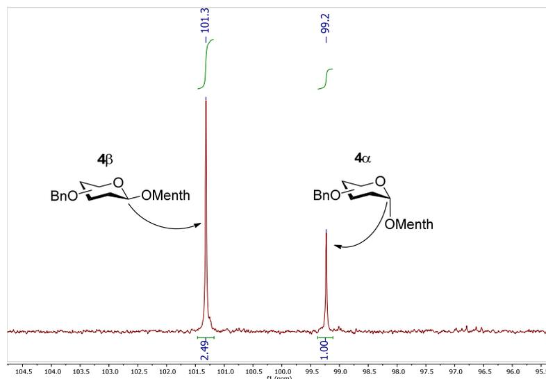
Figure 1.  $^{13}\text{C}$ -NMR spectrum of crude glycosylation mixture showing the signals from the anomeric carbon atoms ( $\beta$ : 101.3 ppm,  $\alpha$ : 99.2 ppm) in  $\text{CD}_3\text{CN}$  of  $4\alpha/\beta$ .
