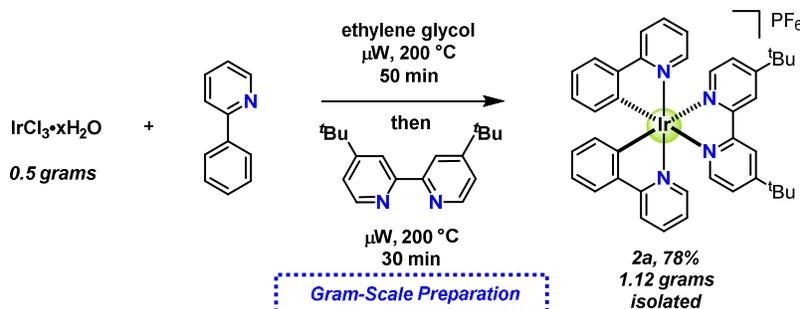
**Scheme 2.** Gram-Scale Preparation of  $[\text{Ir}(\text{ppy})_2(\text{dtbbpy})]\text{PF}_6$ .
