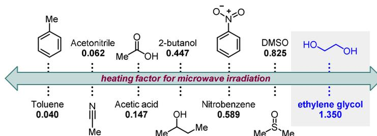
**Figure 2.**  $\tan \delta$  values (heating factor) for common solvents in organic synthesis.
