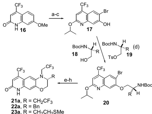
**Scheme 2.** Reagents and conditions: (a) NBS; (b) CsF, *i*-PrI (87% overall); (c) PhSH, NaH, DMF, 110 °C; (d) **19**,  $K_2CO_3$ , or **18**, diisopropylazodicarboxylate,  $PPh_3$ , *N*-methylmorpholine; (e) TFA, EtOAc, 60 °C; (f)  $Pd_2dba_3$ ,  $KOt$ -Bu, BINAP, toluene, 90 °C; (g)  $NaBH_4$ , TFA, 50 °C; (h) HCl/HOAc, 85 °C.
