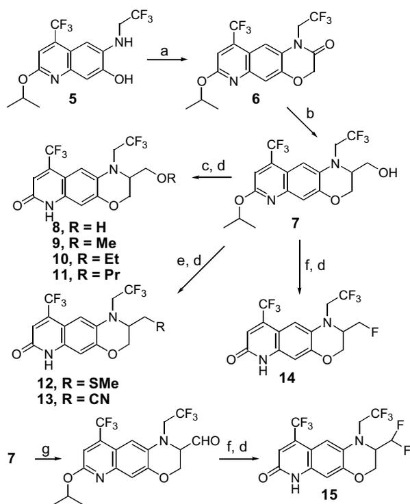
**Scheme 1.** Reagents and conditions: (a) methyl bromoacetate,  $K_2CO_3$ , DMF, 110 °C, 86%; (b) Tebbe reagent, THF, then  $BH_3$ , THF,  $H_2O_2$ , NaOH; (c) NaH, R-I, THF, 0 °C to rt; (d) HOAc:concd. HCl (3:1), 60–80 °C, 75–95%; (e) MsCl,  $NEt_3$ , ether, then NaR, DMF, 80 °C; (f) DAST,  $CH_2Cl_2$ ; (g) Moffatt–Swern oxidation.
