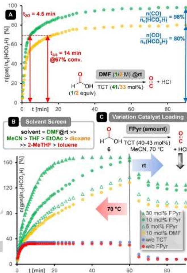
**Figure 1.** Gas volumetry to follow CO formation.  $n(\text{gas})$  = amount of gas as determined by the ideal gas equation,  $n_0(\text{HCO}_2\text{H})$  = initial amount of formic acid, THF = tetrahydrofuran, EtOAc = ethyl acetate, 2-MeTHF = 2-methyltetrahydrofurane.
