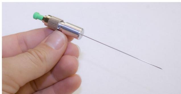
Fig. 2. Imaging needle (diameter 640  $\mu\text{m}$ ).
