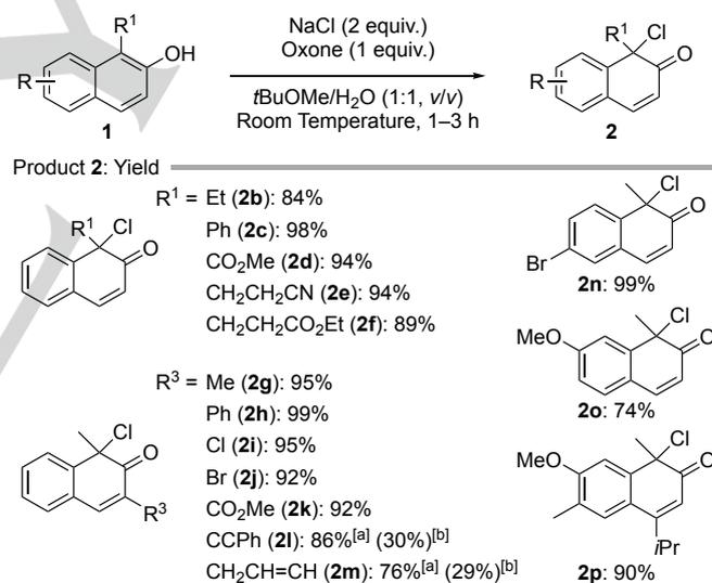
**Scheme 3.** Oxidative chlorinative dearomatization of 2-naphthols **1** with NaCl and Oxone. [a] NaCl (1 equiv.) was used. [b] Reactions were performed under stoichiometric conditions with NaOCl·5H<sub>2</sub>O in AcOH as in Scheme 2.
