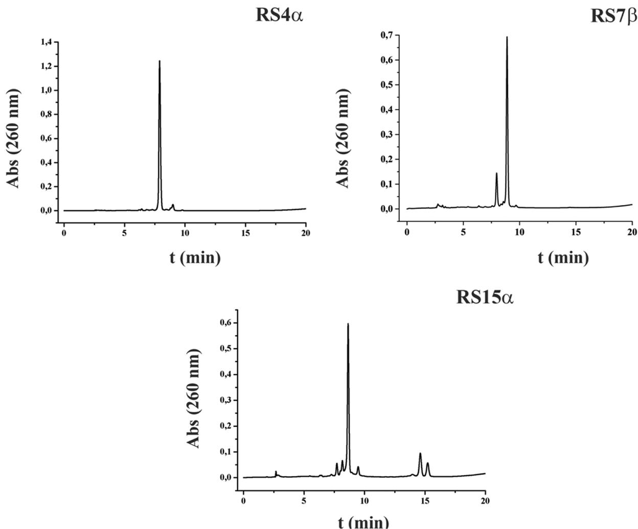
Figure 1. HPLC profiles of model oligonucleotides modified in the 3'-end with 4 $\alpha$ , 7 $\beta$ , and 15 $\alpha$  1,2-dideoxy-D-erythro-pentofuranose derivatives. ACE 3  $\mu$ m HILA-3-1546-A column was used.
