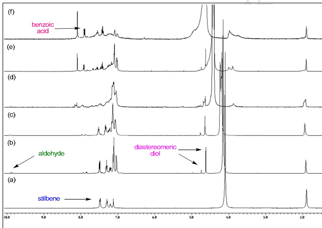
**FIGURE S29.** <sup>1</sup>H NMR monitoring of the oxidation of stilbene in CD<sub>3</sub>CN-D<sub>2</sub>O (1:1) with oxone (5 equiv) at reflux. <sup>a</sup> Before addition of oxone, 0 h, <sup>b</sup> after 2 h, <sup>c</sup> after 4 h, <sup>d</sup> after 10 h, <sup>e</sup> after 20 h, and <sup>f</sup> after 24 h.
