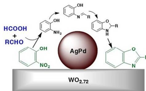
**Scheme 1.** Schematic illustration of one-pot FA dehydrogenation and conversion of nitrophenol/aldehyde to benzoxazole catalyzed by AgPd/WO<sub>2.72</sub>.
