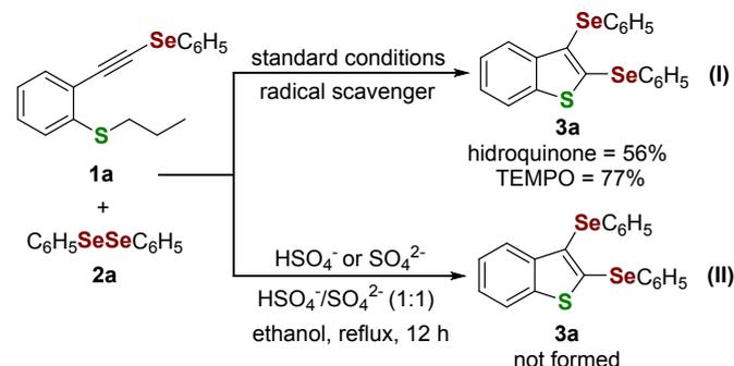
**Scheme 3** Eq. I: Reactions in the presence of radical scavengers; Eq. II: Reactions using the salts present in Oxone<sup>®</sup>.
