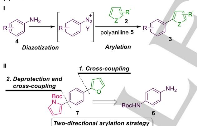
**Scheme 1.** (a) Transition-metal-catalyzed biaryl synthesis, (b) alternative biaryl synthesis via homolytic aromatic substitution, (c) Gomberg-Backmann reaction, (d) previous work, and (e) this work, I: sequential diazotization and arylation, and II: two-directional arylation strategy.
