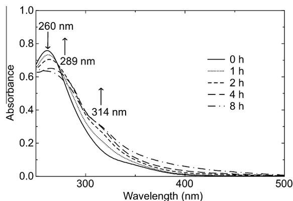
**Figure 3.** UV-vis absorption spectra of **1** irradiated with 365 nm (15 W) in  $\text{CHCl}_3$  ( $[\text{M}] = 1.7 \times 10^{-4} \text{ M}$ ). Spectra recorded at 0, 1, 2, 4, and 8 h.
