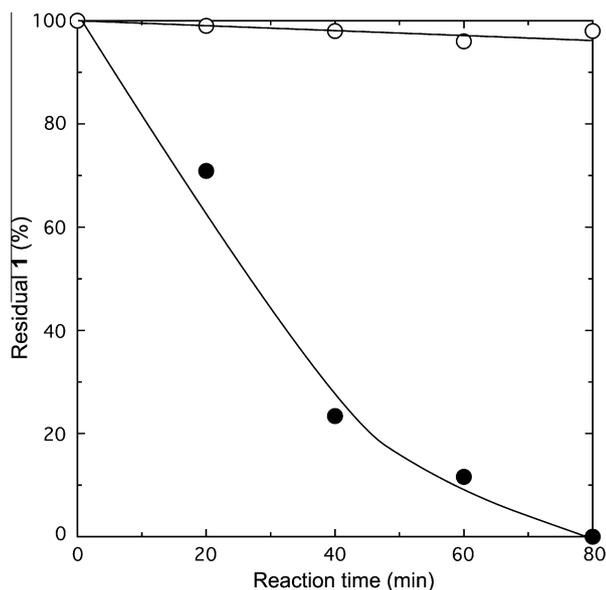
**Figure 1.** Time-course of consumption of **1**. Open circle, in dark; closed circle, irradiated with 365 nm (100 W).
