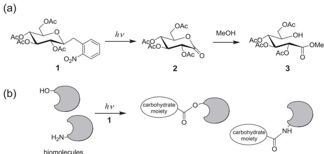
**Scheme 1.** (a) Photochemical conversion of **1**, and alcohol addition to a sugar lactone derivative **2**. (b) Schematic illustration of the reaction of **1** with alcohols or amines in biomolecules.
