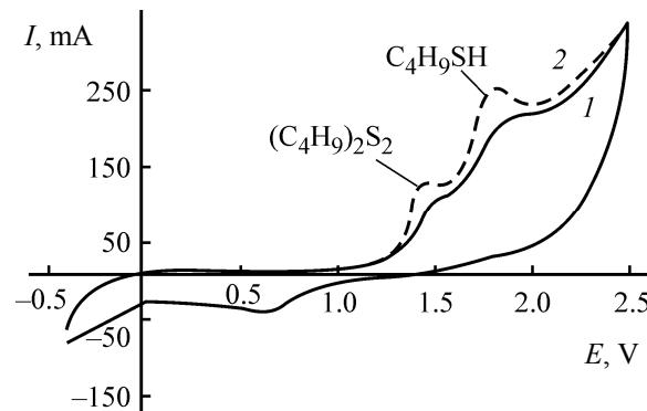
**Fig. 3.** Cyclic voltammogram of the products of electrolysis of  $\alpha$ -butanethiol in (1) **II** and (2) with standard samples (Pt-anode, Ag/AgCl).
