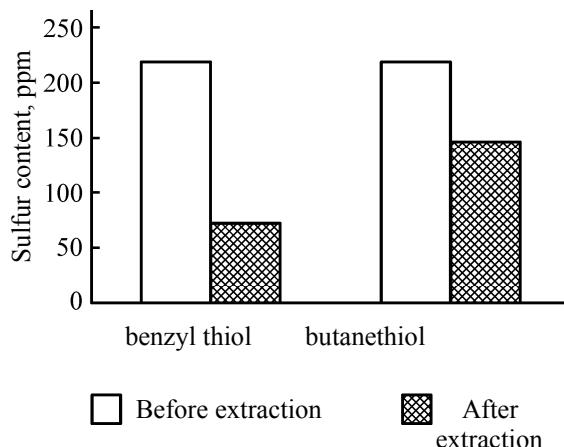
**Fig. 2.** Change of sulfur content in the model hydrocarbon mixtures containing benzyl thiol and butanethiol.
