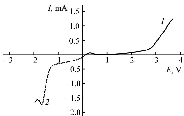
**Fig. 1.** Cyclic voltammogram of the (1) cathode branch (oxidation) and (2) anodic branch (reduction) of **II** (Pt-anode,  $\text{Ag}/\text{AgCl}$ ).
