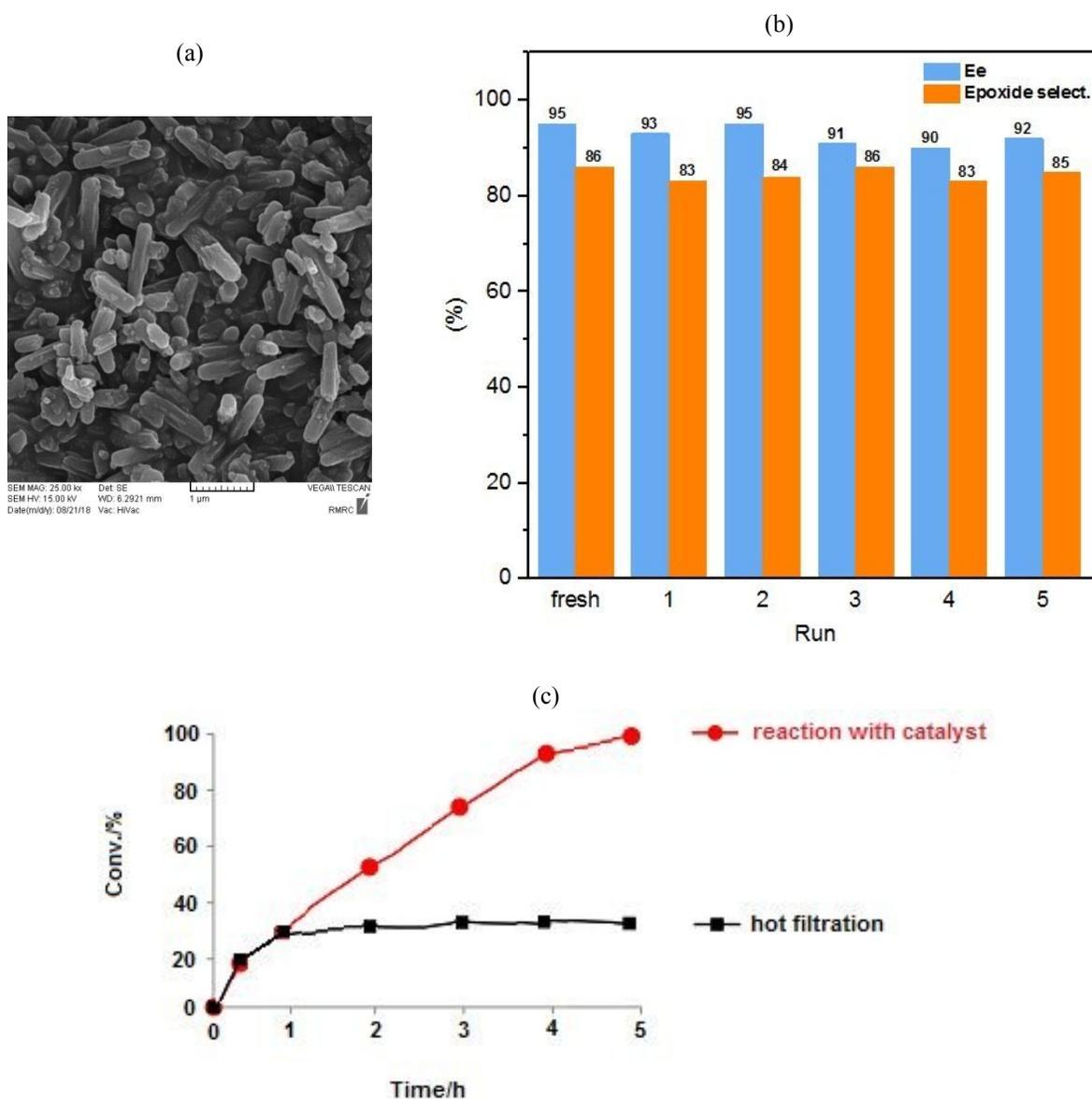
Fig. 5 The SEM image of the used catalyst in the fifth run. The obtained ee and epoxide selectivity by using the reusable [C-NU-1000-Mo] in the oxidation of styrene to five recycles. Hot filtration test was carried out at 80 °C. The epoxidation of styrene with catalyst (red) and after filtering the catalyst from reaction mixture after 1 h (black).
