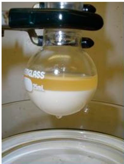
Figure 3. Typical product solution from the treatment of anisole (2 M) with n -BuLi (2 M) with the addition of 0.15 equiv. of TMEDA. The top layer is the supernate and the bottom layer is associated o -LiA precipitate.
