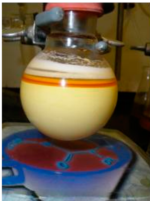
Figure 9. Product solution from treatment of 1.3 M DMBA/1.3 M n -BuLi in cyclohexane containing 1.0 equiv. of MTBE. The top layer is the supernatant and the bottom layer is associated o -LiDMBA.
