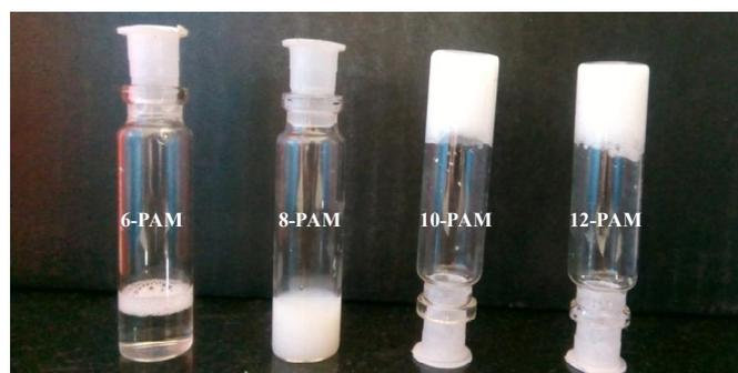
**Fig. 1.** Photograph of vials showing gelation of n-PAM in phosphate buffer solution (pH 8).
