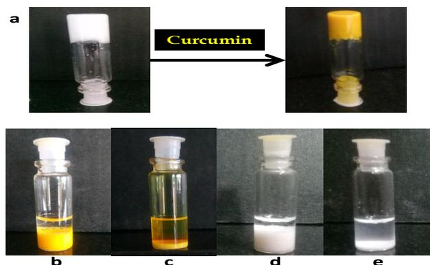
Fig. 6. (a) Visual image of curcumin loaded hydrogel, (b-e) Image showing enzymatic hydrogel degradation in absence and presence of curcumin, (b) curcumin entrapped hydrogel in the absence of enzyme, (c) curcumin entrapped hydrogel in presence of enzyme, (d) hydrogel in the absence of enzyme, and (e) hydrogel in presence of enzyme.
