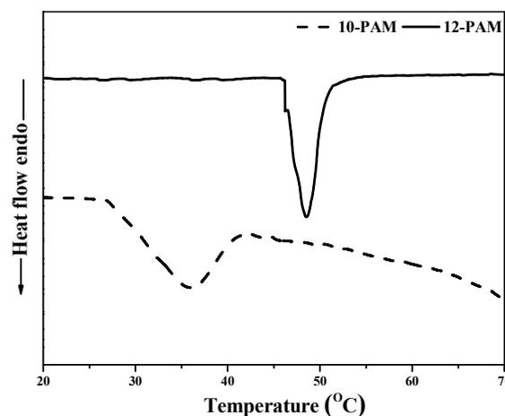
**Fig. 2.** Calorimetric curves of hydrogels.
