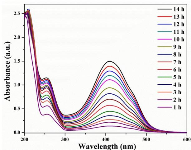
Fig. 7. Absorption spectra of curcumin released from degradation of **12-PAM** hydrogel at different time points 1 to 14h (after 14h absorbance did not increase).
