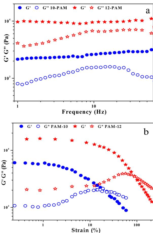
**Fig. 3.** (a) Dynamic frequency sweep rheological experiments for **10-PAM** (1.6 wt%) and **12-PAM** (1.6 wt%) at constant strain of 1%. (b) Dynamic strain amplitude rheological experiment for **10-PAM** (1.6 wt%) and **12-PAM** (1.6 wt%) at constant frequency 1 Hz.
