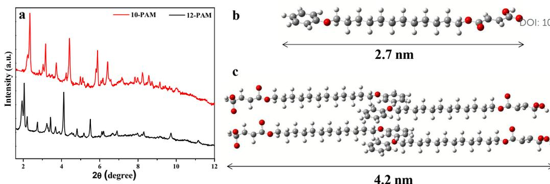
Fig. 5. (a) XRD pattern of the **12-PAM** xerogel, (b) Optimized geometries of **12-PAM** gelator molecule, and (c) Schematic representation of the possible molecular packing models for the **12-PAM** gel.
